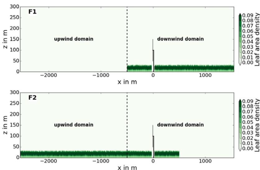
**Figure 1** Sketch of the geometry of the case Case F1 (forest edge upstream of the turbine), case F2 (forest edge downstream of the turbine). Coloured contours mark the leaf area density profiles of the forest with tree heights of 30 m ± 5 m. The wind turbine is placed in a 52 m wide forest clearing at x=0 m, y=0 m. The dashed black line schematically separates the upwind and downwind domain.
