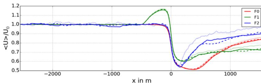
**Figure 3** Scaled u-wind component at hub height ( $z=100$  m) and at  $y=0$  m for the three different cases F0 to F2. Solid, dotted and dashed lines mark corresponding simulations with the wind turbine in MAX, MIN and MEAN position, respectively.
