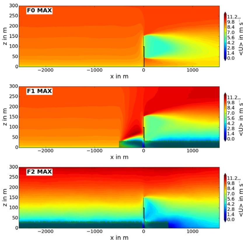
**Figure 2** Vertical cross sections at  $y=0$  m of 30 minute averages of the u-wind component for the F0 to F2 cases with the wind turbine located at the MAX position. The wind turbine is marked with black lines and the forest is indicated with green areas.
