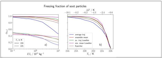
The fraction of emitted soot particles that are activated into ice crystals is displayed as a function of the soot emission index  $El_s$  and the ambient temperature. The various lines show different model configurations. *Taken from Bier et al, 2021*
