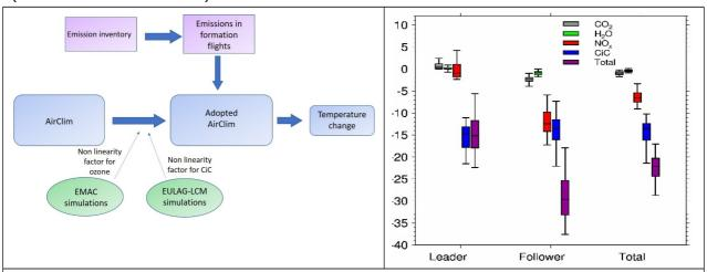
left: Model chain for a comprehensive climate impact assessment of formation flight; right: Change in total climate impact when formation flights are considered. separately for the different species (CiC stands for contrail-cirrus). The bars indicate the 25% and 50% percentile and the whiskers indicate the 95% confidence interval of the different formations in one data set. *Taken from Dahlmann et al; 2020.*
