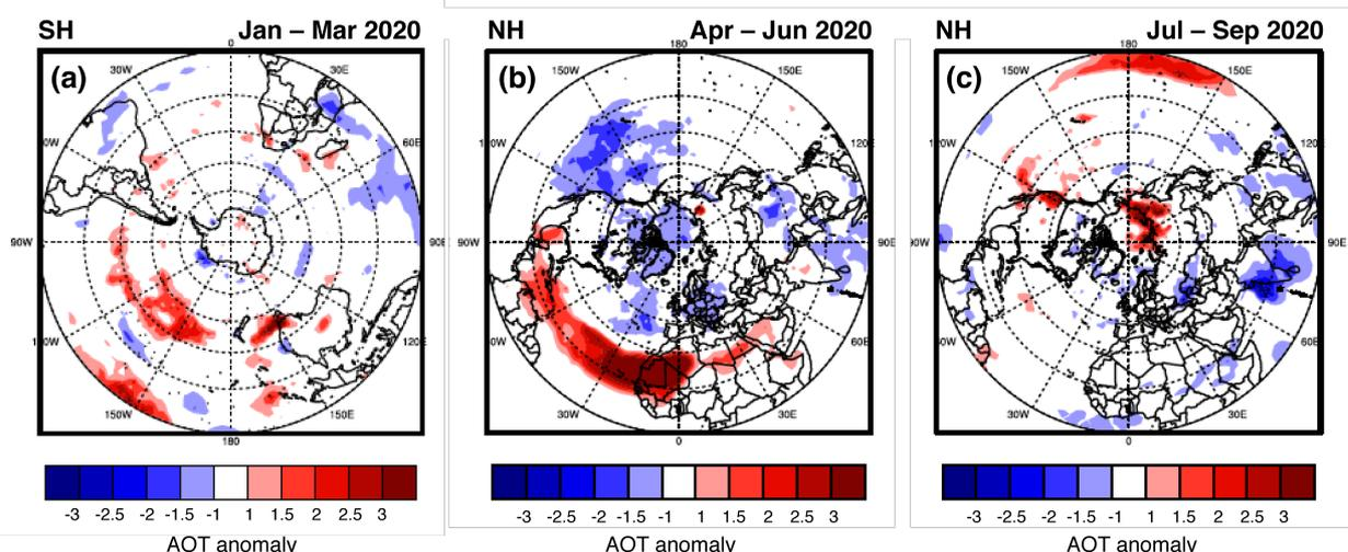
**Figure 1:** Anomalies in monthly mean AOT for 2020 compared to the long-term mean 2010-2019, normalized with standard deviation. The ECHAM6.3-HAM2.3 model results show positive AOT anomalies due to (a) Australia's 'Black Summer' wildfire smoke (Jan-Mar 2020), (b) 'Godzilla' Saharan dust plume (Apr-Jun 2020), and (c) Arctic smoke plume from record Siberian fires (Jul-Sep 2020).
