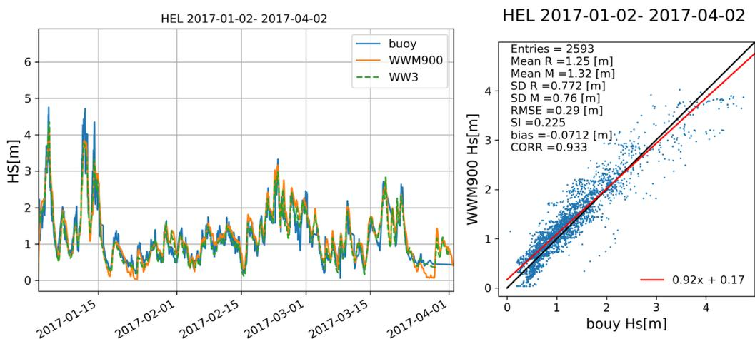
Figure 9: Time Series (left) and scatter plot (right) of significant wave height ( $H_s$ ) simulated by SCHISM-WWM coupled wave model in comparison with buoy data near Helgoland.
