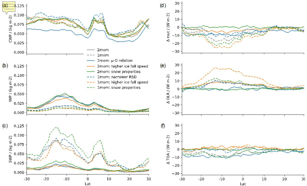
Figure 2: Latitudinal averages of (a) cloud water path (CWP), (b) ice water path (IWP), and (c) snow water path (SWP). Latitudinal average of the difference to the two-moment control run for top-of-the-atmosphere (d) upwelling shortwave radiation, (e) outgoing longwave radiation and (f) the radiative balance.
