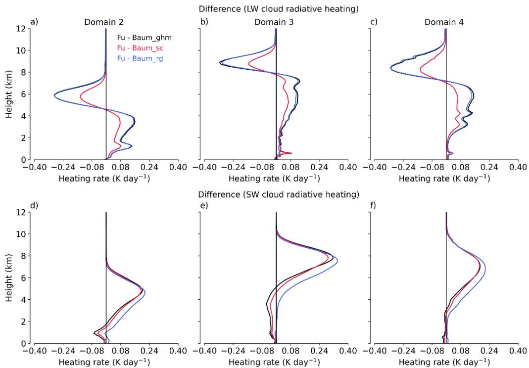
**Figure 3:** Differences in vertical profiles of longwave cloud radiative heating between simulations with the ice optical parametrization of Fu and Baum using different ice habits for domains 2, 3, and 4. The bottom row is for shortwave cloud radiative heating.
