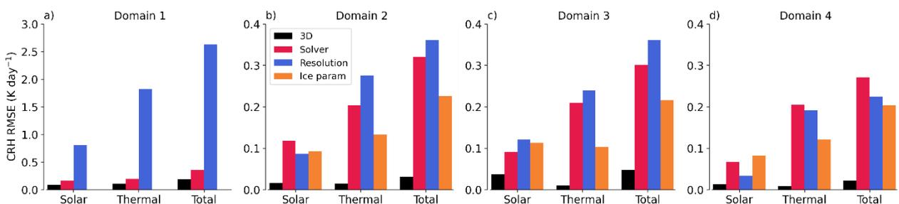
**Figure 2:** Cloud radiative heating uncertainties diagnosed as root mean square error (RMSE) due to 3-d radiative effects (black), radiation solvers (red), resolution (blue), and ice optical parametrization (orange) averaged over the 4 LEM domains.
