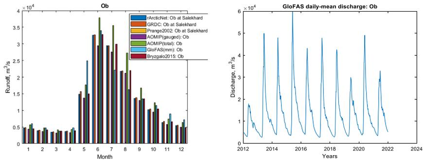
Fig. 1. Left – Climatological monthly-mean river runoff (for the Ob River) as obtained from different sources. Right – Daily-mean river runoff (Ob River) as obtained from the GloFAS.
